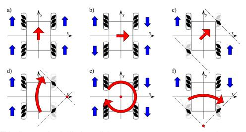
This diagram clearly displays all the necessary ports to move to activate a certain movement, for example going right diagonal would need the top left motor to go forward and bottom right to go forward.
