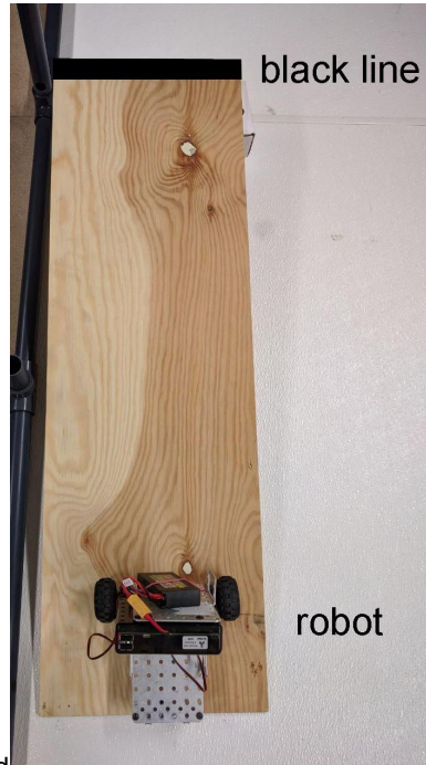
Fig. 1. Robot with the mass mounted at the front, in the starting position on the ramp. The black line indicates the top of the ramp.
