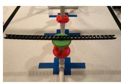
IGUS Chain arm, we can have one motor to extend and retract it as much as we need. The higher we need to go, the more efficient it is. This is also important because our robots have a lot of moving parts, and sparing materials where we can is extremely beneficial for our robots.
