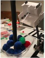
pushes underneath the Poms in the tram and scoops them up, allowing us to keep the design limited to using only one servo. This scooping method is also much more effective at retrieving
