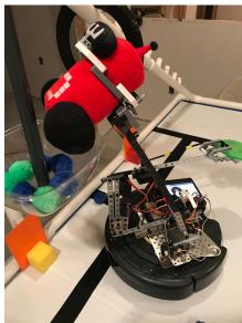
minimizing the weight on the end of the IGUS Chain. Overall, the IGUS Chain apparatus on our large bot is surprisingly useful in grabbing Botguy and putting him in the tram. It uses very little materials and is extremely light and compact, which is less stressful for our servos and motors.
