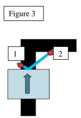
The blue box represents the robot moving towards the right angle turn. The two red dots labeled "1" and "2" represent light sensors.
