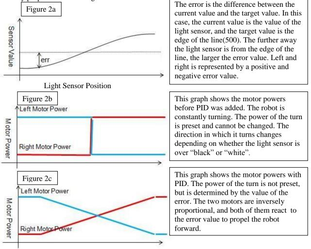
The "Integral" control of PID records the error value over time. If there is a consistent pattern to the errors, then the robot will compensate for it. For example, if the robot is constantly drifting to the left, the program will add a slight right turn in order to counteract the unwanted movement. Lastly, the "Derivative" portion of the program will predict the next error. It does this by subtracting the previous error and the current error.
