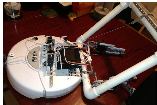
Figure 5: Finalized iRobot Create design
