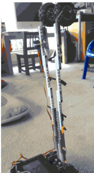
Figure 3: Arm design more compact robot design. However, we decided against that design because of a lack of servos, the likely complexity of programming to control such a jointed robot arm, and the weight of the arm.
