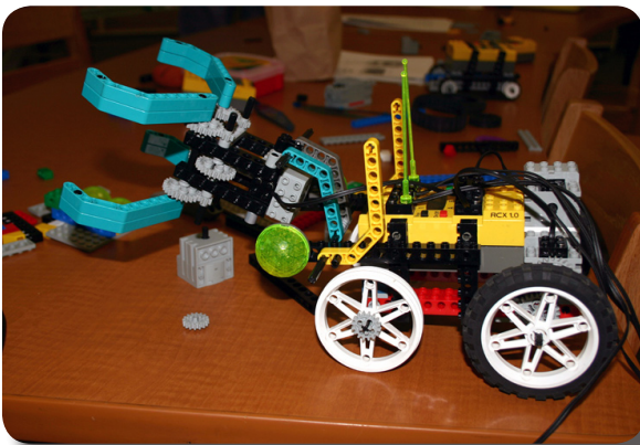
Figure 2: Modification of Tank Bot with Wheels and a Claw
