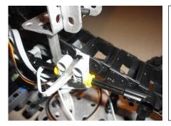
This is where the sensor sends a signal and the KIPR Link tells the motor at the front section of the robot to stop turning.
