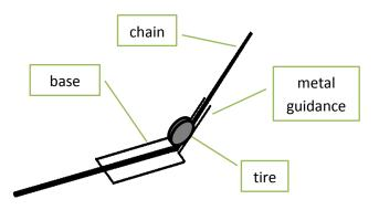
guidance is in)! The next thing we had to come up with a solution for was the fact that the chain of course didn't ROLL up itself, but acted like a solid bar after a downward movement, as you can see on the schematic drawing above.
