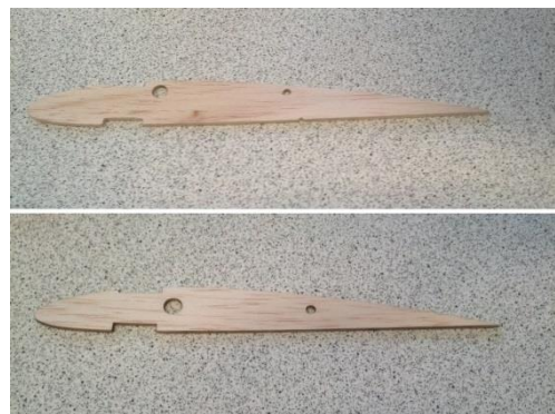
Figure 8: Comparison of milling (top) and laser cutting (bottom). Milled frame had to be grinded after milling. Laser cut frame has burned but sharp edges.
