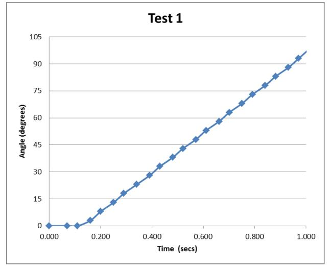
This graph explicitly shows that there is a period of time where no movement is recorded. (The actual inactivity is 0.1401 seconds). This information facilitates the prediction of when to stop the iCreate. Coupled with the how much overshoot there is, turning based on time has become a much easier endeavor. Testing different speeds yields similar delay periods, but different overshoot degree values. By adding:
