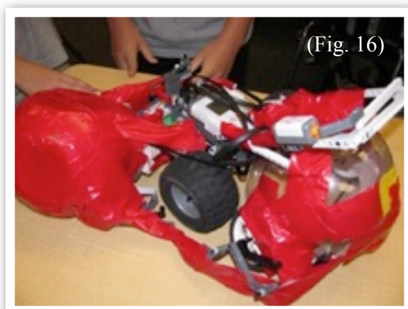
This is a NXT lawn mower. The original design might just be a toy, but the student modified it to be able to sweep up the tribbles used in Botball. It moves along mowing the tribbles into the catcher bins. (Fig. 16)
