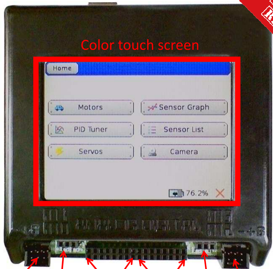
2 servo motor ports 2 motor ports 8 analog sensor ports 8 digital sensor ports 2 servo motor ports 2 motor ports
